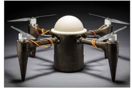
Figure 2 | CRACUNS can be launched from a fixed position underwater or from an unmanned undersea vehicle. Image courtesy of Johns Hopkins Applied Physics Laboratory.
