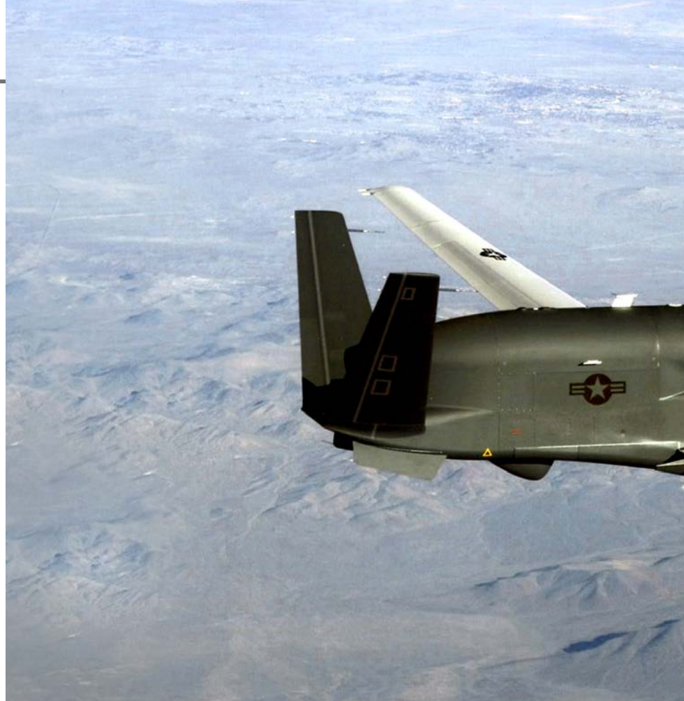
An RQ-4 Global Hawk unmanned aerial system (UAS) soars through the sky to record intelligence, surveillance, and reconnaissance data. (Air Force courtesy photo.)
